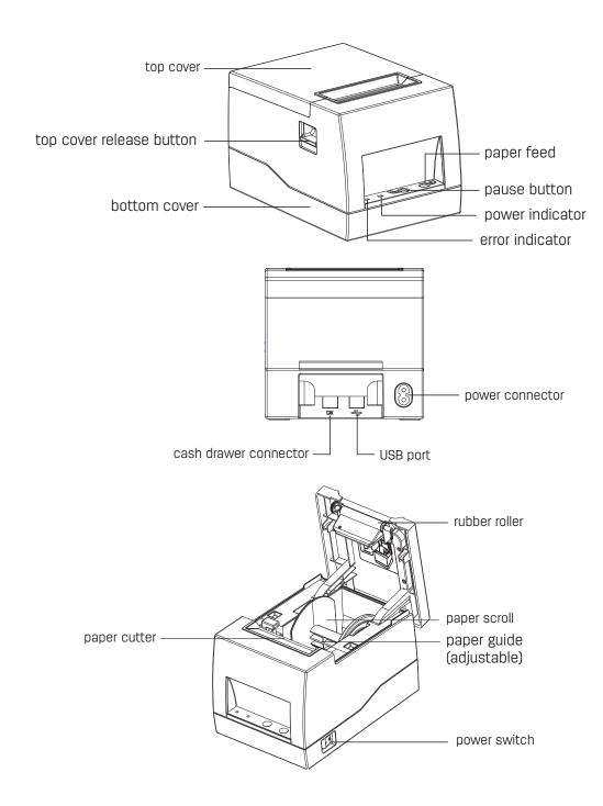
Note: Keep your fingers away from the paper cutter while printing, or you may cut your finger. The company shall not be liable for any injury caused by the paper cutter during operation.
