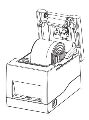
5. Pull out part of the paper roll through the paper guide, and close the paper guide according to the paper width to regulate both sides of the paper.
