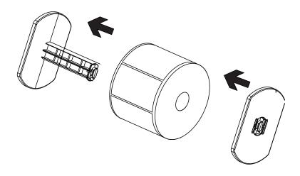
4. Load the paper roll set into the printer from top to bottom.
