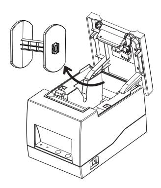
3. Pull out the paper roll stopper to the right and load the paper roll. Fix the paper roll with the paper roll stopper according to the roll paper width.
